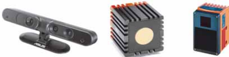
Figure 1: Devices used in this work. On the left an Asus Xtion Pro Live, a Mesa SR 4000 in the centre and an IFM O3D200 on the right.
