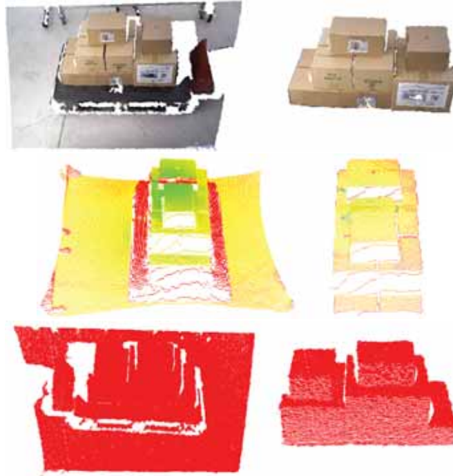
Figure 14: Processing example for a point cloud acquired by the Asus Xtion Pro Live, Mesa SR 4000 and Asus Xtion Pro respectively. The first picture of each pair is the point cloud acquired directly and the second the result of the segmentation process, where only the merchandise remains.
