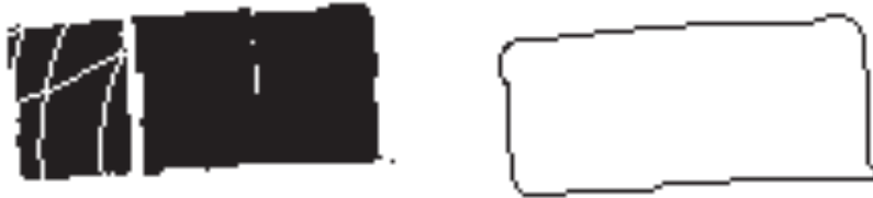
Figure 18: The left picture corresponds to a top view of the point cloud shown in Fig. 17 after projecting the two upper planes onto the plane below (the three planes of this merchandise have been projected, so all points have the same height). On the right, it is displayed the same picture after being processed applying a dilating and an eroding filter, then a Gaussian filter and afterwards the canny edge detector. The area of the plane is computed through this image.
