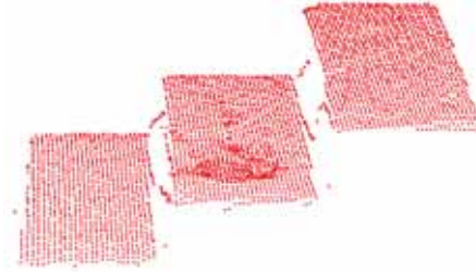
Figure 17: Mesa's point cloud acquired from the top of the arch, depicting a zenithal view. This configuration of the merchandise corresponds with the case 14 of Fig. 19 and consists of three columns of boxes with different heights.
