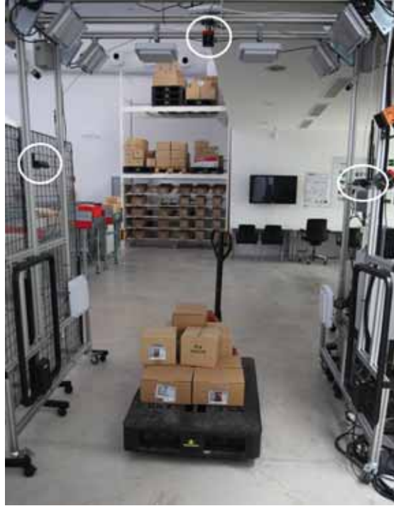
Figure 12: Configuration chosen for the devices. Both Asus on the sides and the Mesa on the top part. The Asus registers lateral information exclusively and the Mesa gives an upper view of the scene, being its z -axis perpendicular to the floor plane. The cameras have been highlighted in the image with white circles.
