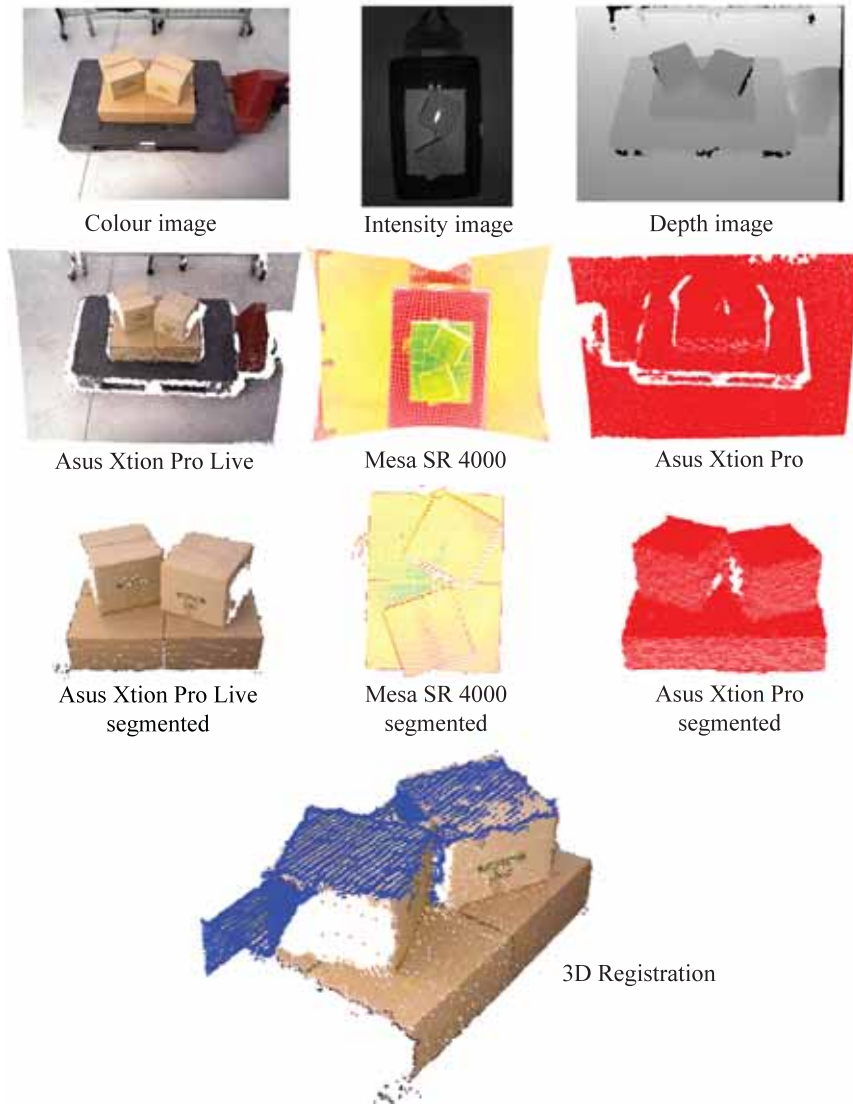
Figure 21: Summary of the intermediate steps for the volume estimation process in the case 9. The first row corresponds with the raw image acquired by the devices. The second row is the same image after being transformed into a point cloud. The third row represents the point cloud after being segmented, that is to say, only the merchandise remains. Finally, the last point cloud is the result of doing a 3D registration with the segmented point clouds. Starting from this point cloud, the final step is the volume computation of the merchandise through the application of the designed algorithms.
