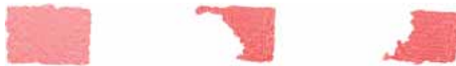
Figure 11: On the left, an Asus' point cloud of a card. In the other two images, the same card when the Asus works with an IFM simultaneously. The holes in the two latter are a consequence of interferences caused by IFM.
