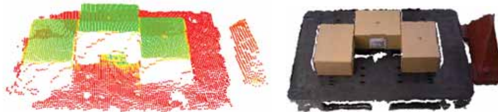
Figure 15: Instance of two point clouds where there are reflections. In both the floor has been extracted previously. On the left, it can be noticed a Mesa’s point cloud with a reflection in the pallet (green points which should be red) caused by the own camera. On the right, a point cloud taken by the Asus Xtion Pro Live simultaneously which is not affected by this phenomenon.
