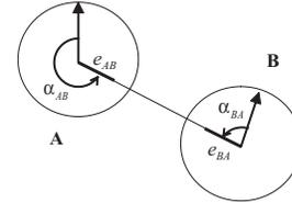
Fig. 1. Nomenclature and conventions used throughout the paper.  $e_{AB}$  is the epipole (i.e. the projection of the optical center) of view B in view A.  $\alpha_{AB}$  is the angle or direction of that epipole, i.e. its angular polar coordinate in view A. The reference axis for the measurement of the angles is the robot's axis of orientation (the vertical axis of the images). The angles are measured counterclockwise and are defined between  $-\pi$  and  $\pi$ .
