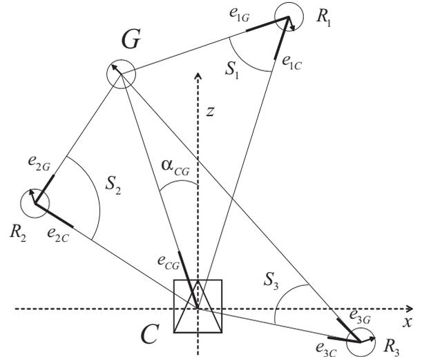
Fig. 5. Elements involved and angles employed in the homing strategy.  $C$  is the robot's current localization, at the coordinate origin  $(0, 0, 0)$ .  $G$  is the goal location.  $R_i$  are reference views. Three of the  $n$  views on the reference set are depicted as example.
