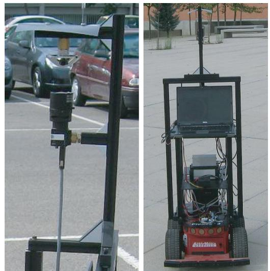
Fig. 9. Omnidirectional camera (left) and complete setup (right) used for the first indoor experiment and the outdoor experiment.
