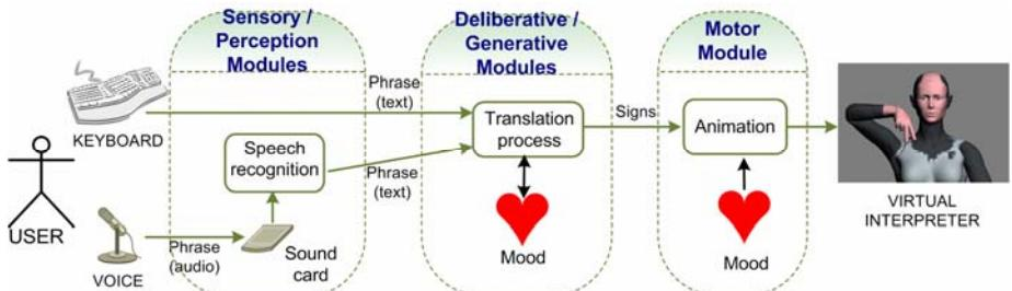
**Fig. 2.** Integration of the translation tool in the animation engine
