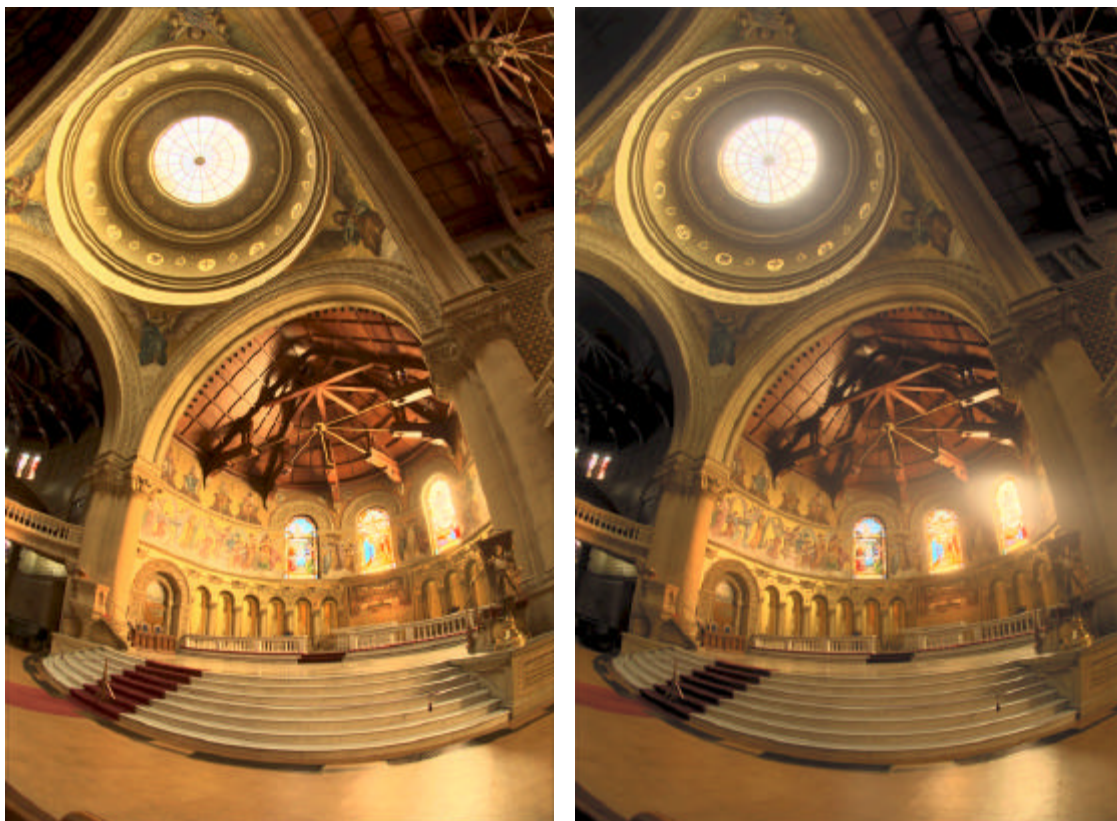
Fig. 3. On top, the workflow of SEKER. Bottom, two tone mapped HDR images; left: only tone mapped, right: tone mapped and simulation of contrast sensitivity, color loss, veiling glare and visual acuity loss.
