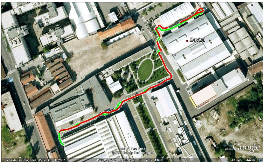
Figure 2.14: GPS trajectory (red) and SLAM trajectory (green) superposed on the satellite image of the Campus of Bovisa (Milan) where the sequences were acquired
