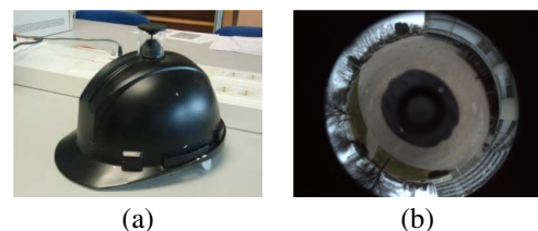
Figure 1. (a) Helmet-camera device. (b) Omnidirectional image captured with this device.
