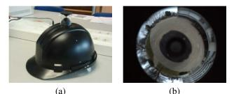
Fig. 1: (a) Hemlet-camera device used in our experiments. (b) Omnidirectional image captured with our device.
