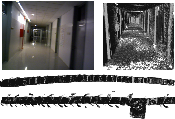
Fig. 6. (Top-left) RGB image of the corridor, (Top-right) pcl KinFu 3D reconstruction with our visual odometry method, (middle) side view and (bottom) plant view of the complete 3D mesh. Note the challenging of the sequence due to the poor texture of the corridor and light reflexes.
