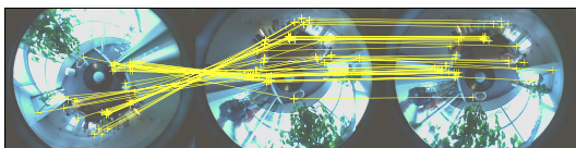
Figure 1: Omnidirectional image: feature extraction and matching.
