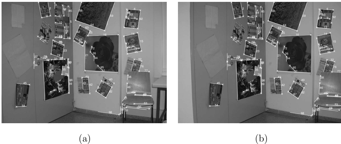
Fig. 8. Computation of matches in image pair of nearly null baseline. The features all over the image are explained with only one homography.
