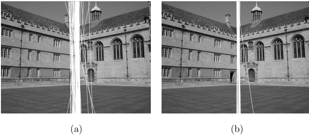
Fig. 4. Intersection lines of two planes through the eigenvalues of the homology. The lines corresponding to one hundred runs are represented without the homology filter (a) and with it (b).
