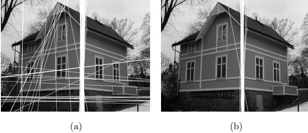
Fig. 3. Intersection lines of two planes through the eigenvalues of the homology. The lines corresponding to one hundred runs are represented without the homology filter (a) and with it (b).
