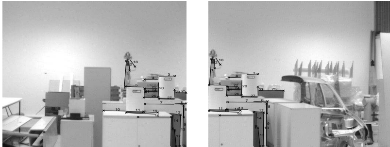
Fig. 1. Images showing the final matches when the robot rotates 18 degrees. Only one match is no good (10), which is a wrong match as segment although good as line.
