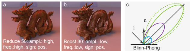
Figure 11: a and b . Results of gloss editing using [BBPA15], making the material less and more shiny, respectively (the parameters used are specified in the figure, for their meaning please refer to [BBPA15]). c . Illustration of these operations on an input reflectance lobe (purple), as it is made more shiny (green) or less shiny (blue). Solid lines correspond to the ground truth, and dashed ones to the results obtained by scaling the lobe.
