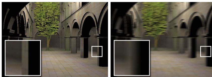
Fig. 17. Simulation of hold-type blur [222]. A user is shown the same animation sequence (sample frame on the left) simultaneously at two different refresh rates. The subject's task is to adjust the blur in the sequence of the right (120 Hz) until the level of blur matches that of the sequence on the left (60 Hz). The average result is shown here: the blurred sequence on the right displayed at 120 Hz is visually equivalent to the sharp sequence on the left displayed at 60 Hz (image copyright Wiley 2010).
