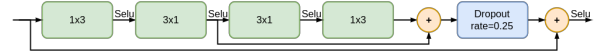
Fig. 4. Convolutional module: Four separable convolutions with two residual connections. Lastly a dropout layer is applied to help dealing with overfitting.
