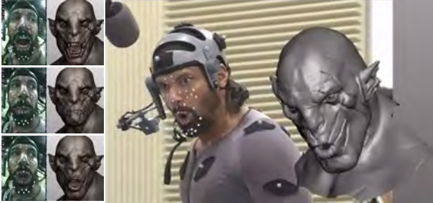
Figure 3. Motion capture system applied to films. Left: Several selected frames used to recover facial expressions by means of artificial markers. Right: A multi-camera system is used to track the motion of the face or object. The recovered motion is augmented with virtual objects performing a realistic trajectory. Images copyright Weta Digital.
