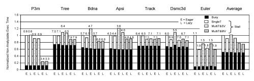
Fig. 17. Supporting architectural main memory (AMM) schemes in a CMP. In the figure, E and L stand for Eager and Lazy, respectively.
