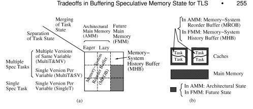
Fig. 6. Buffering and managing speculative memory state: taxonomy (a) and difference between architectural (AMM) and future main memory (FMM) schemes (b).
