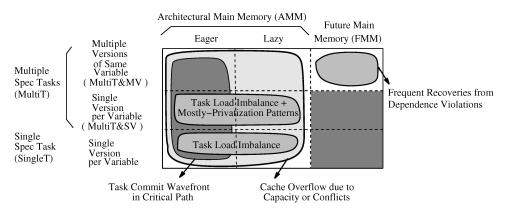
Fig. 12. Application characteristics that limit the performance of our schemes.
