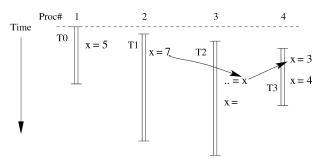
Fig. 2. Multiple versions of the same variable in the system. The figure shows examples of in-order RAW, out-of-order WAR, and WAW dependences.
