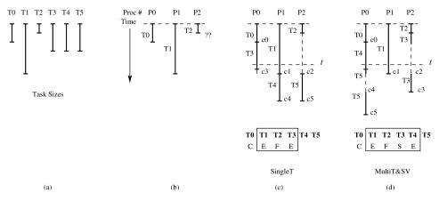
Fig. 14. Example in *Tree* where MultiT&SV is slower than SingleT. Charts (c) and (d) also show the status of the tasks at time t, where C, E, F, and S stand for committed, executing, finished, and stalled.
