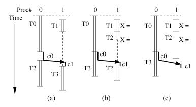
Fig. 9. Four tasks executing under SingleT (a), MultiT&SV (b), and MultiT&MV (c).
