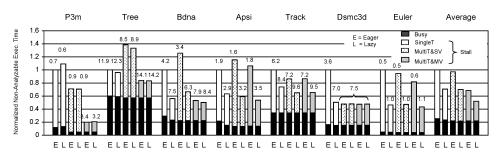
Fig. 13. Supporting single or multiple speculative tasks or versions per processor, for eager or lazy architectural main memory (AMM) schemes. In the figure, *E* and *L* stand for Eager and Lazy, respectively.
