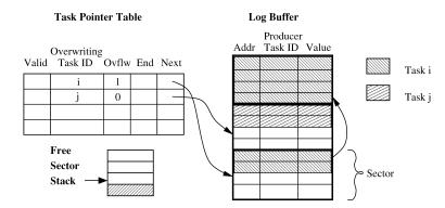
Fig. 18. Per-processor software structures that we use to implement the software MHB in FMM.Sw.  $\,$
