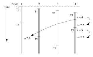
Fig. 4. External request to a cache that has two versions of the same variable *x*.
