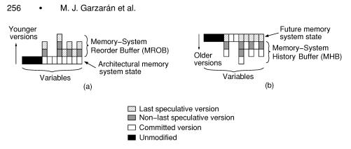
Fig. 7. Snapshot of the memory system state of a program under TLS using the concepts of Memory-System Reorder Buffer (a) and Memory-System History Buffer (b).
