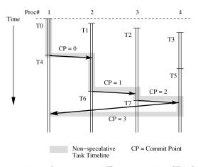
Fig. 1. A set of tasks executing on four processors. The commit point (CP) advance is shown in the nonspeculative task timeline.
