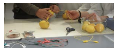
Figure 4: Experiment performed by the High School students at Centro Universitario de la Defensa: Generating electricity with basic elements: a lemon, a nail and a coin.
