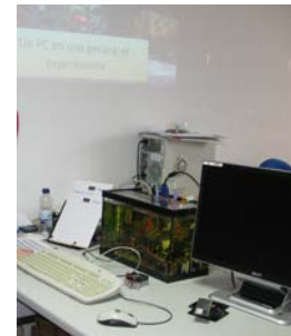
Figure 3: Experiment performed at the computer architecture lab, a PC is used in a fishbowl to explain how heat dissipation plays an essential role in computing devices.
