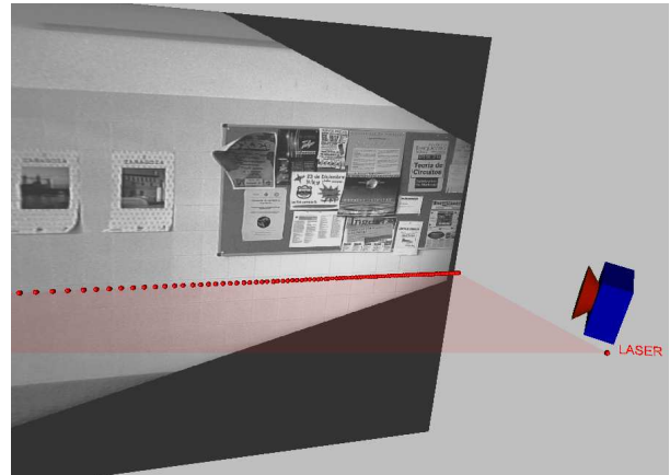
Fig. 1. The combination of complementary sensors allows the use of highly descriptive observations. The subsequent identification of corresponding features between the measurement and the map is therefore greatly simplified.
