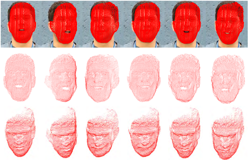
Figure 4: Face sequence: dense 3D point cloud estimation. Top: Selected frames #17, #43, #55, #75, #100 and #121 with 3D reprojected mesh. Middle: Original viewpoint. Bottom: General view.
