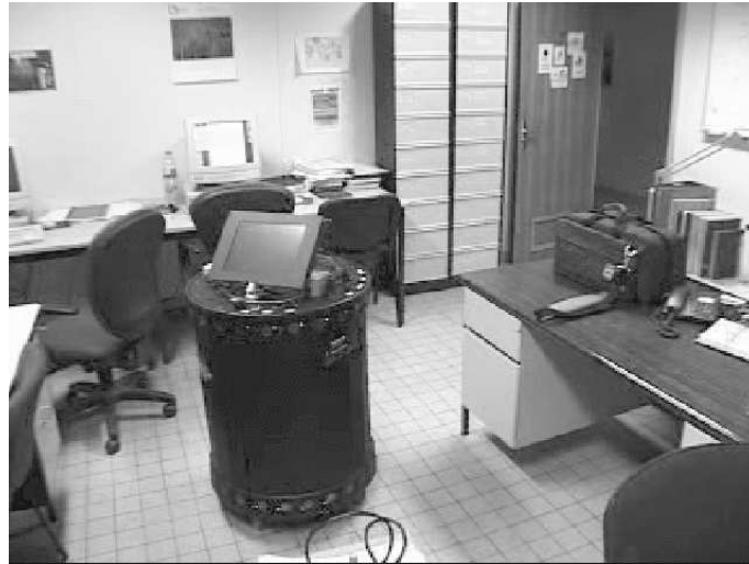
Figure 2.1: Typical office environment. The snapshot was taken in a experiment performed using the Robels system. The Nearness Diagram Navigation is the sensory-motor function that is driving the robot out of the office.
