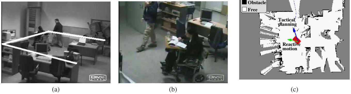
Fig. 2. These figures show the wheelchair moving in the office environment and the model computed with the planner and reactive method solution at a given time. (a) Moment when the trap situation was produced; (b) Moment when the wheelchair performs the avoidance of the chair on the path and the moving obstacle. (c) Model constructed and the solutions of the tactical planner and the reactive method.
