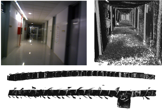
Figure 12: (Top-left) RGB image of the corridor, (Top-right) KinectFusion 3D reconstruction with our visual odometry method, (middle) side view and (bottom) plant view of the complete 3D mesh. Note the challenging of the sequence due to the poor texture of the corridor and light reflexes.
