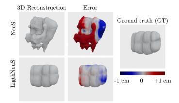
**Fig. 2. Benefits of illumination decline**. Result on the "*Cecum 1 a*" sequence. **Top:** The NeuS reconstruction exhibits multiple artifacts that make it unusable. **Bottom:** Our reconstruction is much closer to the ground truth shape. The error is shown in blue if the reconstruction is inside the surface, and in red otherwise. A fully saturated red or blue denotes an error of more than 1cm and grey denotes no error at all.
