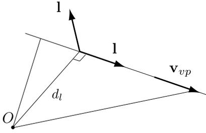
Figure 1: Components of a Plücker description of a 3D line. The direction vector  $\mathbf{l}$  and the moment vector  $\bar{\mathbf{l}}$ . Under Manhattan World assumption a main direction  $\mathbf{v}_{vp}$  is coincident with the direction  $\mathbf{l}_i$  of lines following this direction and orthogonal with their moment vectors  $\bar{\mathbf{l}}_i$ .
