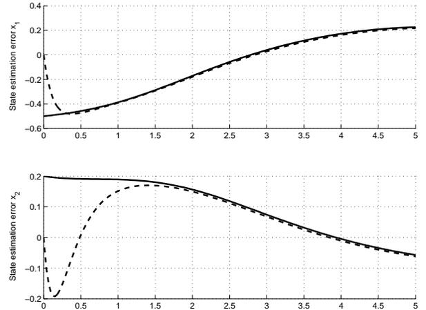
Fig. 1. Estimation results of the state variable. From top to bottom, state estimation error  $\tilde{x}_1(t)$ ,  $\tilde{x}_2(t)$ .
