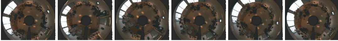
Fig. 10. Sequence of some images taken by the robot camera during an experiment. The first is the target image, the second is the initial and the last is the image at the end of the motion.
