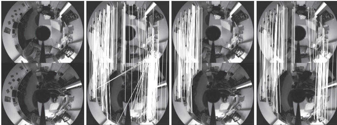
Fig. 7. Example of two images ( 1^{st} column). Putative SIFT matches ( 2^{nd} column). Point correspondences left after homography estimation with standard method ( 3^{rd} column) and using the multiple homography approach ( 4^{th} column).
