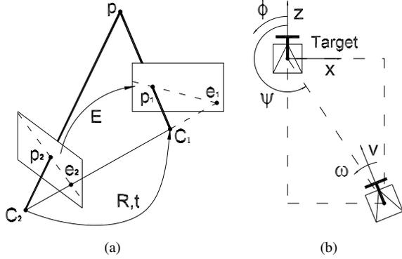
Fig. 2. (a) Essential matrix relating two views. The camera optical centers are  $C_1$  and  $C_2$ . A 3D point  $P$  is projected in the images as  $(p_1, p_2)$ . The epipoles are  $e_1$  and  $e_2$ . (b) Coordinate system fixed in the target location.
