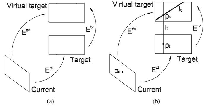
Fig. 3. (a) Essential matrices across the views. The virtual target is defined above the target. (b) A 3D point is projected into the three views as  $(p_c, p_t, p_v)$ . The value of  $p_v$  is computed by means of the epipolar transfer.
