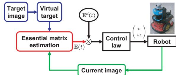
Fig. 1. Overview of the control loop.
