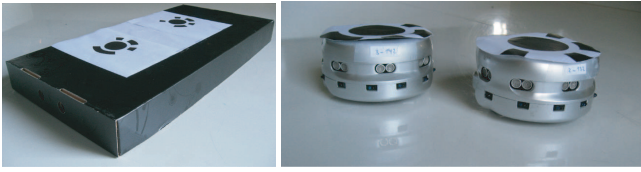
Fig. 11 Box shaped object (left) and the two khepera robots (right).
